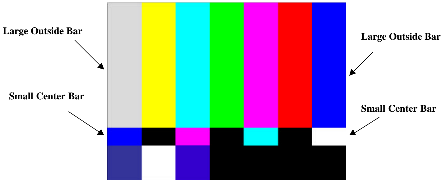
Fig 4: The SMPTE bar pattern blue and white bars are used to calibrate the television color control.
